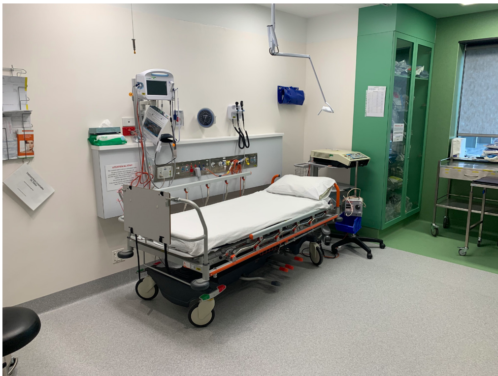
Fig 1. Minor procedure room containing 12-lead electrocardiogram and monitor, wall suction and oxygen, pneumatic trolley, LED procedural light, bipolar diathermy, tourniquet machine, hand table, set-up trolley, gown trolley, infrared activated scrub sink, 99 per cent alcohol surgical hand rub and storage cupboards for consumable equipment
